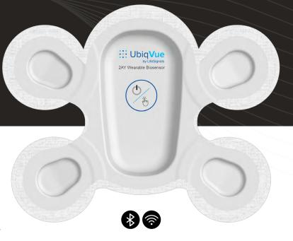
Featuring the all-in-one, chest-worn UbiqVue 2AY Biosensor, patients can move freely within a hospital or home setting. Their biodata are continuously captured and transmitted in near real-time<sup>1</sup> for up to 5 days.
